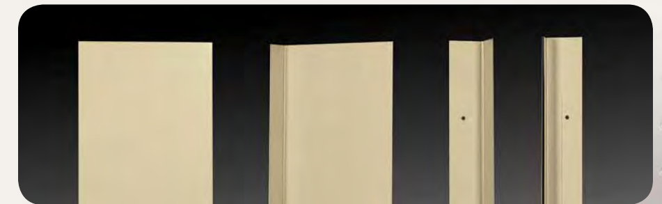
Angle Filler Panel/Flat Filler Panel Angle filler panels are used to close the space between a locker and the wall or between two lockers when an obstruction prevents the installation of another locker. Flat filler panels require two filler panel frames; angle filler panels require only one.
