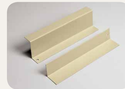
Z Brace/Bottom Angle Z Braces provide reinforcement and secures the bottom of the locker to the floor, while adding toe-space under the locker. Bottom angles are used as a decorative filler for the bottom face of the locker.
